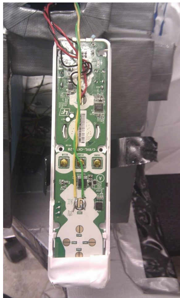
Fig. 5. Wires soldered onto the Wiimote.
